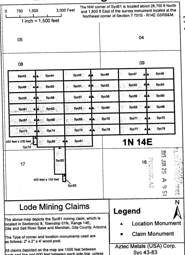
each end line and 600 feet between each side line, unless otherwise noted. The bearings between all claim corners are
